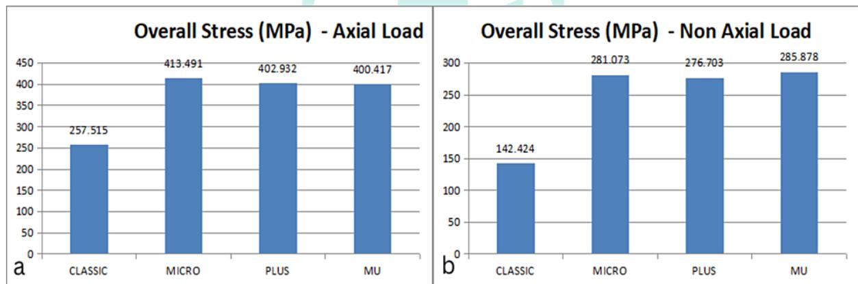
Fig. 5 Overall stress a) Axial load b) Non axial load
